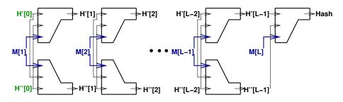
Fig. 3. The Double-Pipe Hash
