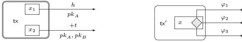
Fig. 1. (Left) \text{tx} is published on the blockchain. The output of value x_1 can be spent by a transaction containing a preimage of h and signed w.r.t. pk_A . The output of value x_2 can be spent by a transaction signed w.r.t. pk_A and pk_B but only if at least t rounds passed since \text{tx} was accepted by the blockchain. (Right) \text{tx}' is not published yet. Its only output can be spent by a transaction whose witness satisfies \varphi_1 \vee \varphi_2 \vee \varphi_3 .
