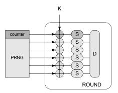
**Fig. 3.** Simplified view of one round in AES Rijndael. The counter feeds a particular sequence of messages to the device. PRNG is a pseudo-random generator producing arbitraty message sequences. K is the encryption key, S denotes an s-box and D is the diffusion layer of the round.
