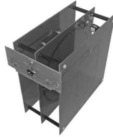
Fig. 2. Helmholtz assembly according to ISO/IEC 10373-6
