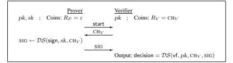
Fig. 3. Reset-secure identification protocol  $\mathcal{ID}$  for the CR1 setting based on a deterministic, stateless digital signature scheme  $\mathcal{DS}$ .
