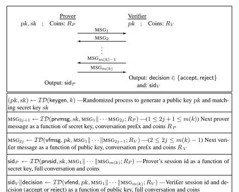
Fig. 1. The prover sends the £rst and last messages in an m(k)-move identification protocol at the end of which the verifier outputs a decision and each party optionally outputs a session id. The *protocol description* function  $\mathcal{ID}$  specifies all processes associated to the protocol.
