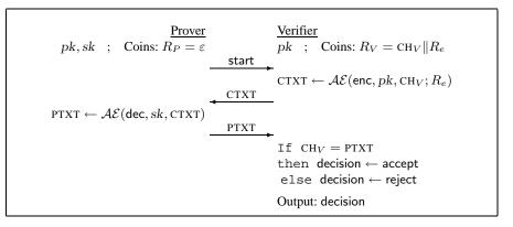
Fig. 4. Reset-secure identification protocol  $\mathcal{ID}$  for the CR1 setting based on a chosen-ciphertext attack secure asymmetric encryption scheme  $\mathcal{AE}$ .
