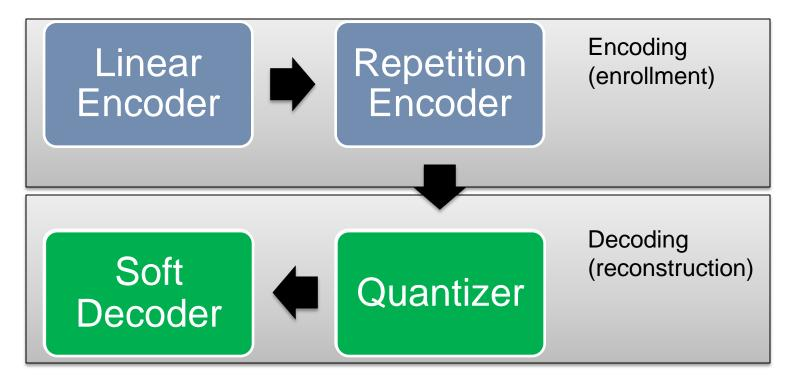
• Quantizer: only a single enrollment measurement required
