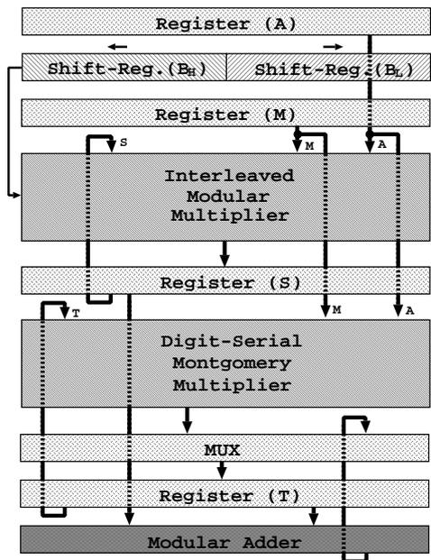
Fig. 3. Block diagram of a multiplier
