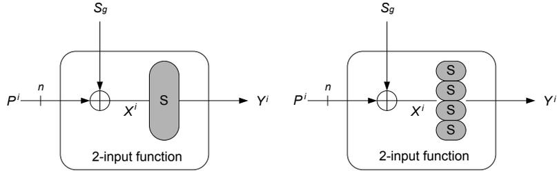
Fig. 2: Single block and multiple block cipher implementation.
