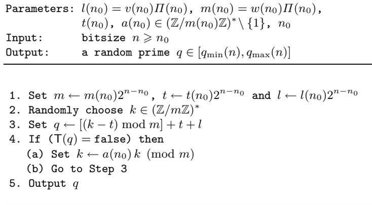
**Fig. 5.** Our scalable prime generation algorithm.
