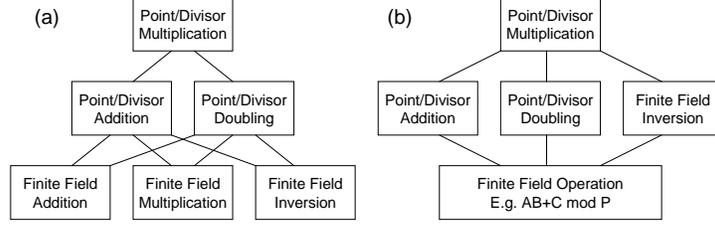
**Fig. 1.** Scheme of the hierarchy for ECC/HECC operations.
