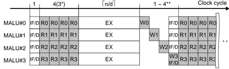
**Fig. 4.** Example of four parallel issue of instructions in case of allocating four MALUs. (IF/D: Instruction Fetch/Decode, EX: Execution of MALU, R/W: Read/Write from/to the coprocessor memory). \*The read cycle differs from the type of operation. \*\*The write cycle depends on the number of instructions issued in parallel.
