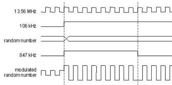
**Fig. 8.** noisy modulation of the sub-carrier
