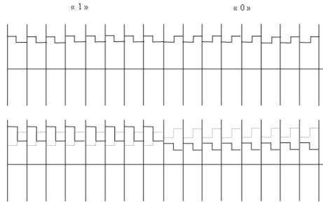
**Fig. 5.** Above: 2 bits of a tag answer (bit rate 106 kbits), Below: The noise added synchronized with the tag answer (bit synchronized) as it could be seen with a probe in the field. We can notice that the noise is not specific to a "1" or "0" and that its phase and amplitude are varying.
