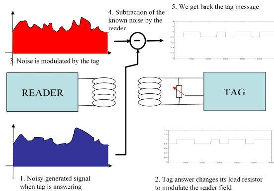
**Fig. 1.** The principle of the noisy reader. First, the reader generates a noisy signal and emits it through its antenna during the period of the tag answer. Secondly, the tag, in order to answer, modulates its load as any other tag. So the reader or a spying probe in the field will see a noisy signal where the tag message is hidden. But, as the reader knows the noise it emitted, it can subtract it from the signal it received to retrieve the tag message.
