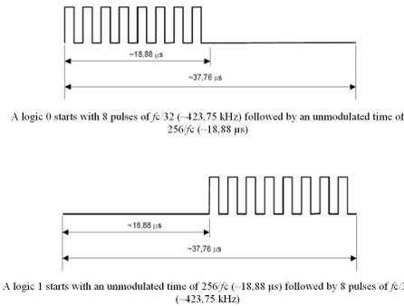
**Fig. 2.** Type A bit coding of the card reply
