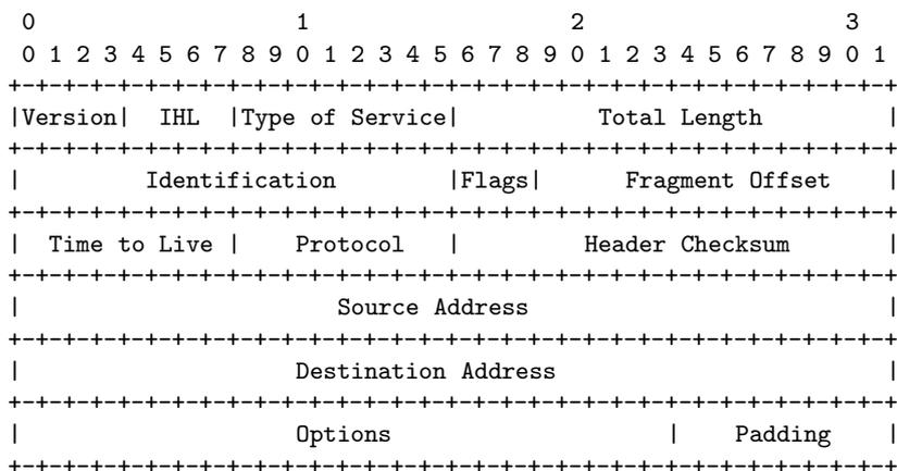
**Fig. 1.** Structure of IP header according to RFC 791, [20].
