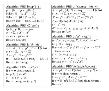
**Fig. 10.** The partially blind signature scheme  $PBS = PBS[\mathbb{G}]$ .
