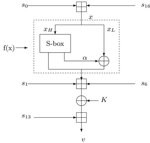
**Fig. 1.** The non-linear filter of SOBER-32 without stuttering
