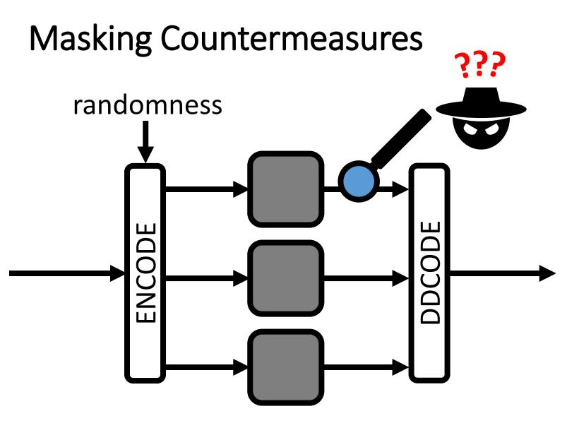
Data is encoded to multiple shares. Unable to get data only by probing a wire.
