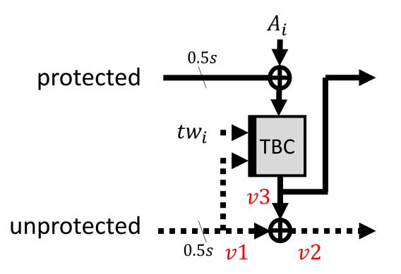
The protected value v3 is recovered from unprotected values v1 and v2.
