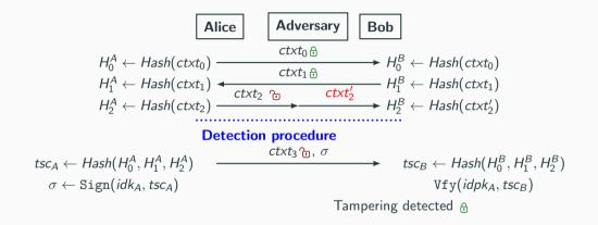
Transcripts sent in the authentication step are authenticated with long-term keys. In this example,  $H_2^A \neq H_2^B$  so the attacker is detected in-band.
