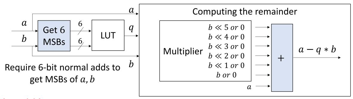
$\lfloor \log_2(6) \rfloor + 1 = 3$  CSA delays
