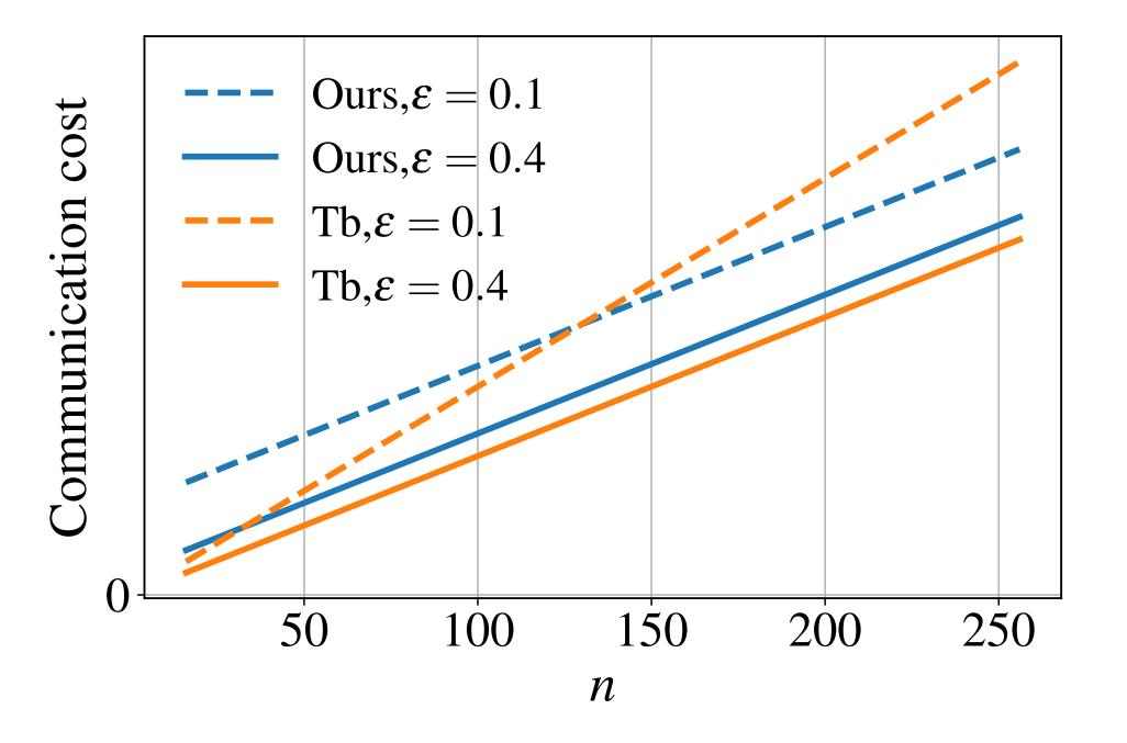
SuperPack has advantage for small  $\epsilon$  and large n. The ratio of Turbospeedz / SuperPack is between 0.83 and 1.6. The cost is reasonable considering the performance gain during online phase.
