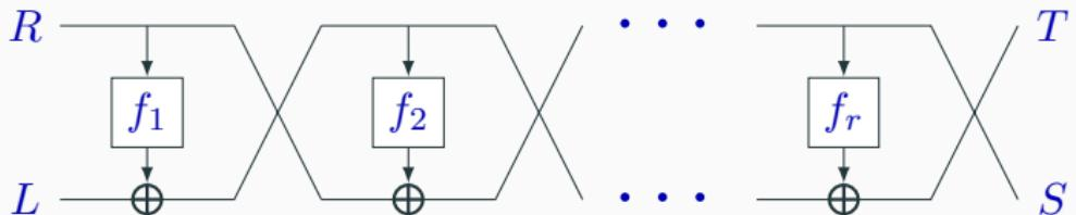
Most security analyses are done in Random Oracle model: for  $F_1, \dots, F_r \leftarrow \$\text{Func}(n)$ ,
