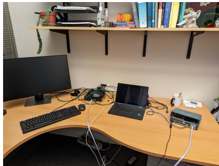
PoC with Cisco ASA 5505 firewall tunneling UDP via TCP to our cluster.
