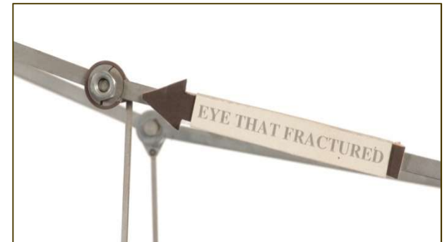
Image from model of bridge (credit: NIST)
